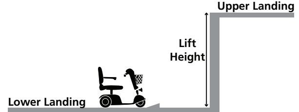
Floor installation = Floor to floor distance
